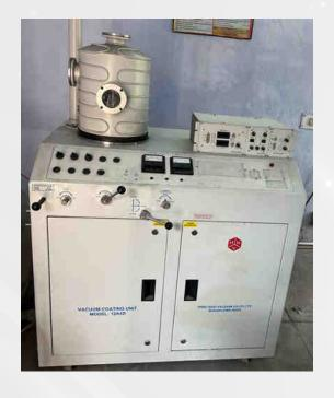
Equipment 12: Electron Beam Physical Vapour Deposition (EBPVD)
